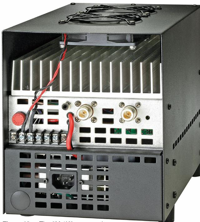
Figure 12 — The 6M-1K2 rear panel.
